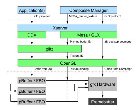
Figure 4: Xgl in combination with a composite manager
